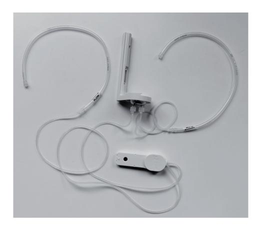
Picture of a gamma-irradiated BioConnect, with C-flex and dead plugs instead of Male Luer locks.
