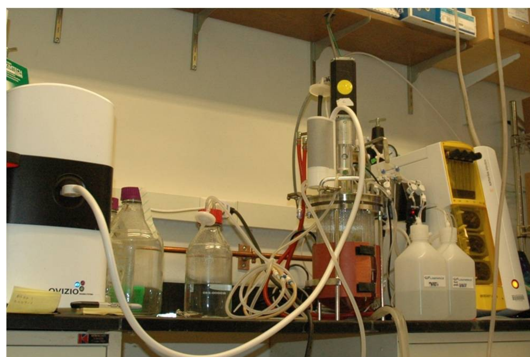
Figure 1. Bioreactor Set Up - To the extreme left is the in-line microscope (Iline F-Ovizio Imaging Systems, Belgium) connected to the reactor through a fluidic system (BioConnect - Ovizio Imaging Systems, Belgium). To the extreme right is the control tower (Sartorius Stedim, Germany) of the bioreactor.
