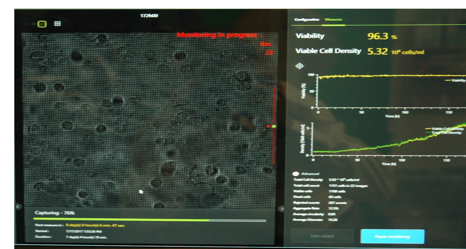
Figure 5. Screen capture from the In-line Microscope on seventh day of the run- The picture is a screen capture from the monitor of the computer attached with the in-line microscope, in the center of the screen is the images of the cells as viewed by the in-line microscope and towards the right are the cell density and the viability trends observed by the software along with additional information on cell size and culture parameters.
